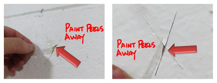
The manufacturer will determine if the substrate is acceptable if the tape pulls up the paint. We are also looking for a chalky film under the paint and or the primer, <u>which will likely be a reason for rejection.</u>
